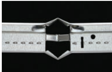
Main beam exposed to fire
