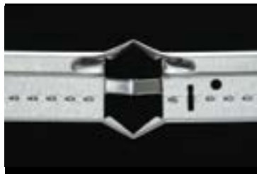
Main beam exposed to fire
